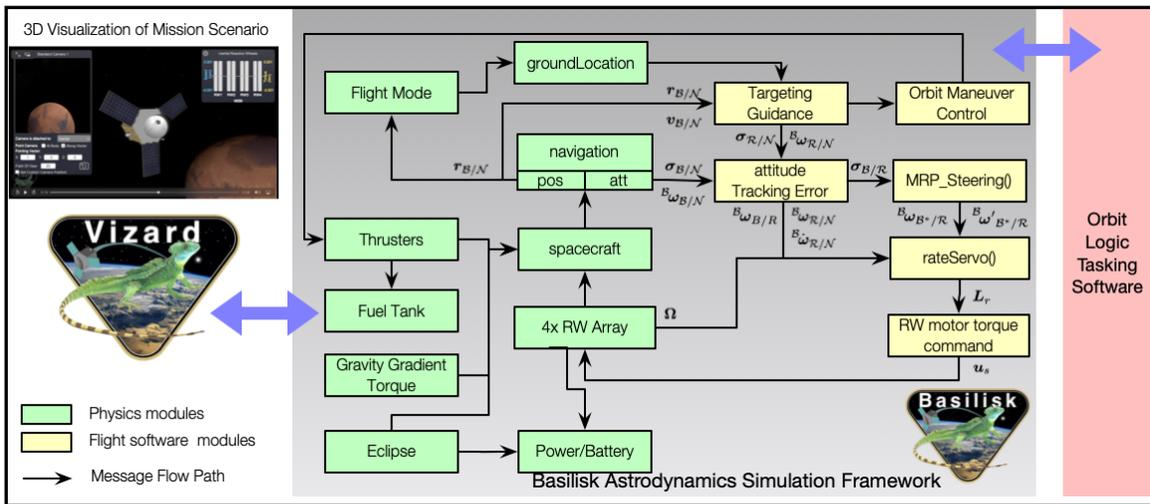
Figure 3. Basilisk Simulation Workflow for Commanded Pointing and Maneuvering.
