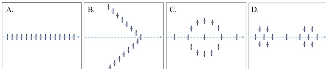
**Figure 1. Several prototypical satellite orbital flight formation configurations, such as A. leader-follower, B. staggered swept echelon, C. and D. circular-projected and leader-follower combinations.**
