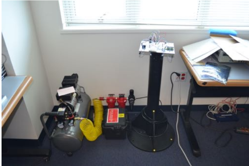
Figure 3.3: Image of the air bearing testbed in the GNAT Lab at NASA Ames Research Center. The test craft with IMU sensor spins on the air bearing while the visual attitude system images onboard LEDs and computes the attitude. Yellow markers on the air bearing allow us to transform to an inertial frame.
