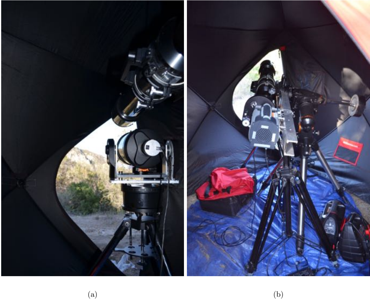
Figure 7.11: (a) shows the guide telescope ( bottom ) and science telescope ( top ). (b) shows the science telescope with EMCCD mounted on the back. The EMCCD and the electronics are powered by battery packs.
