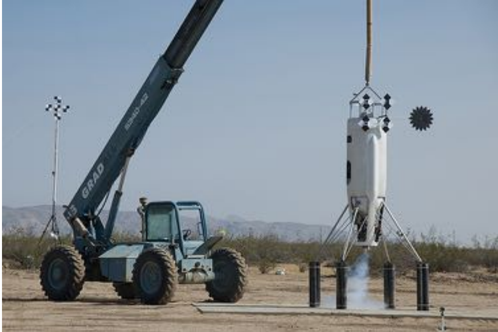
Figure 4.1: Masten Space System's Xaero-B is seen tethered on the launchpad with our payload attached. The tall structure in the background are visual targets used as a reference when calculating the motion of the vehicle using camera data. Image credit: NASA.
