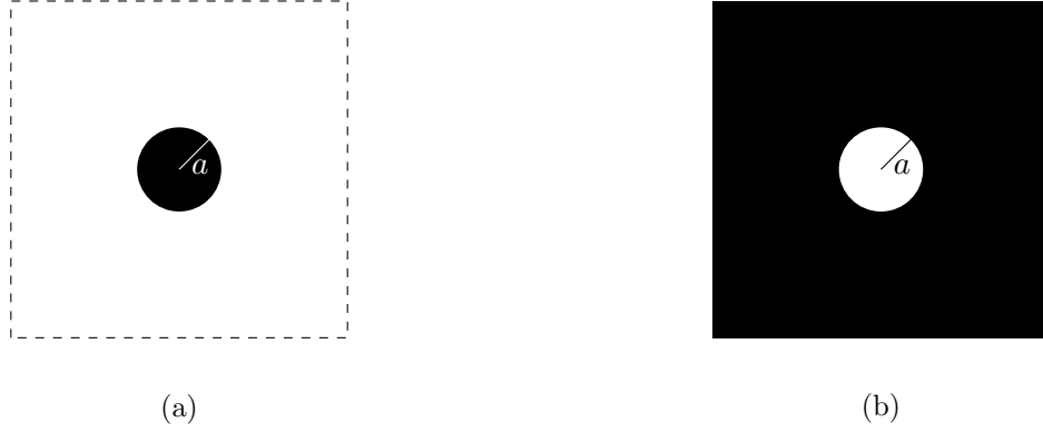
Figure 2.5: (a) is the screen for which we are trying to calculate the diffraction pattern. (b) is the complementary screen that we use to solve the integral. Babinet's Principle states that the sum of the electric fields of the two screens are equal to the field that would exist if neither screen were present.
