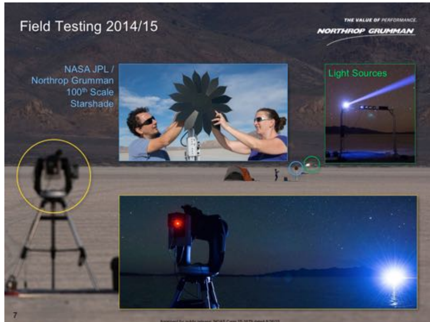
Figure 6.8: Images from the Northrop Grumman-led project field testing starshades on dry lake beds. The telescope is circled in yellow , the 60 cm starshade, located 1 km away is circled in blue , and the light source, located an additional 1 km away is circled in green . (Taken from [90])
