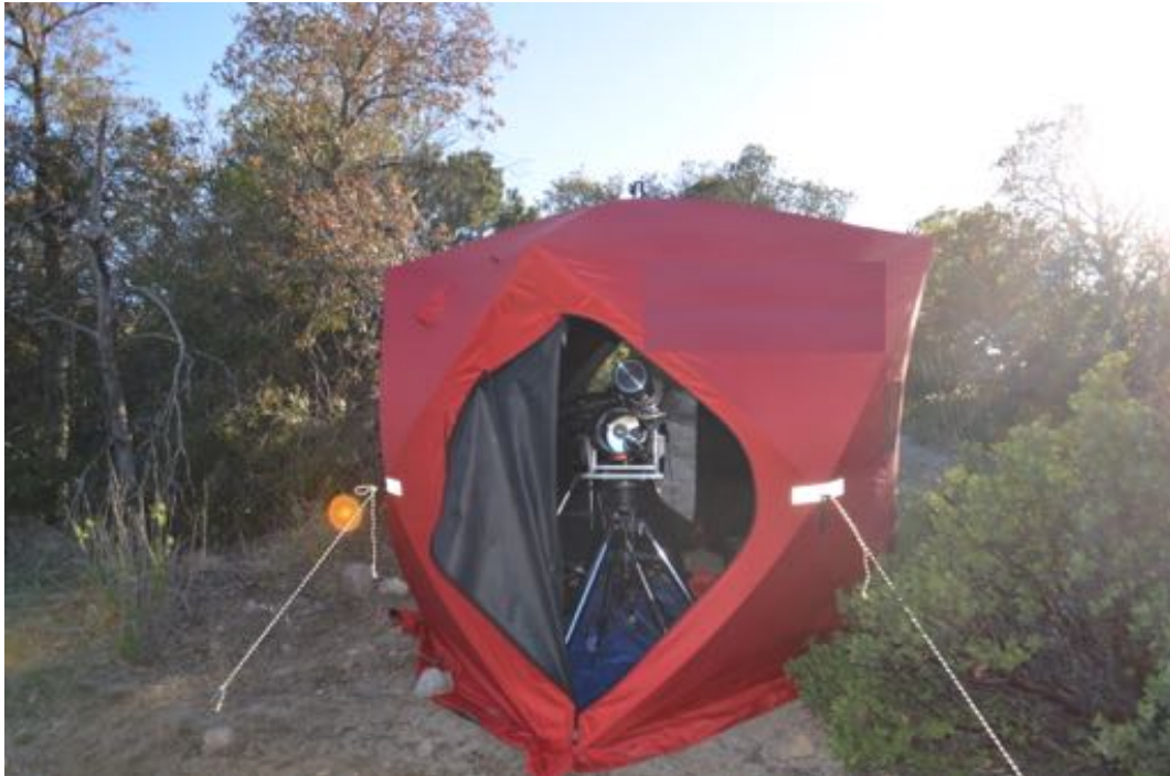
Figure 7.10: Image of telescope tent. The top telescope is the 12.7 cm science telescope, the bottom telescope is the 15 cm guide telescope.
