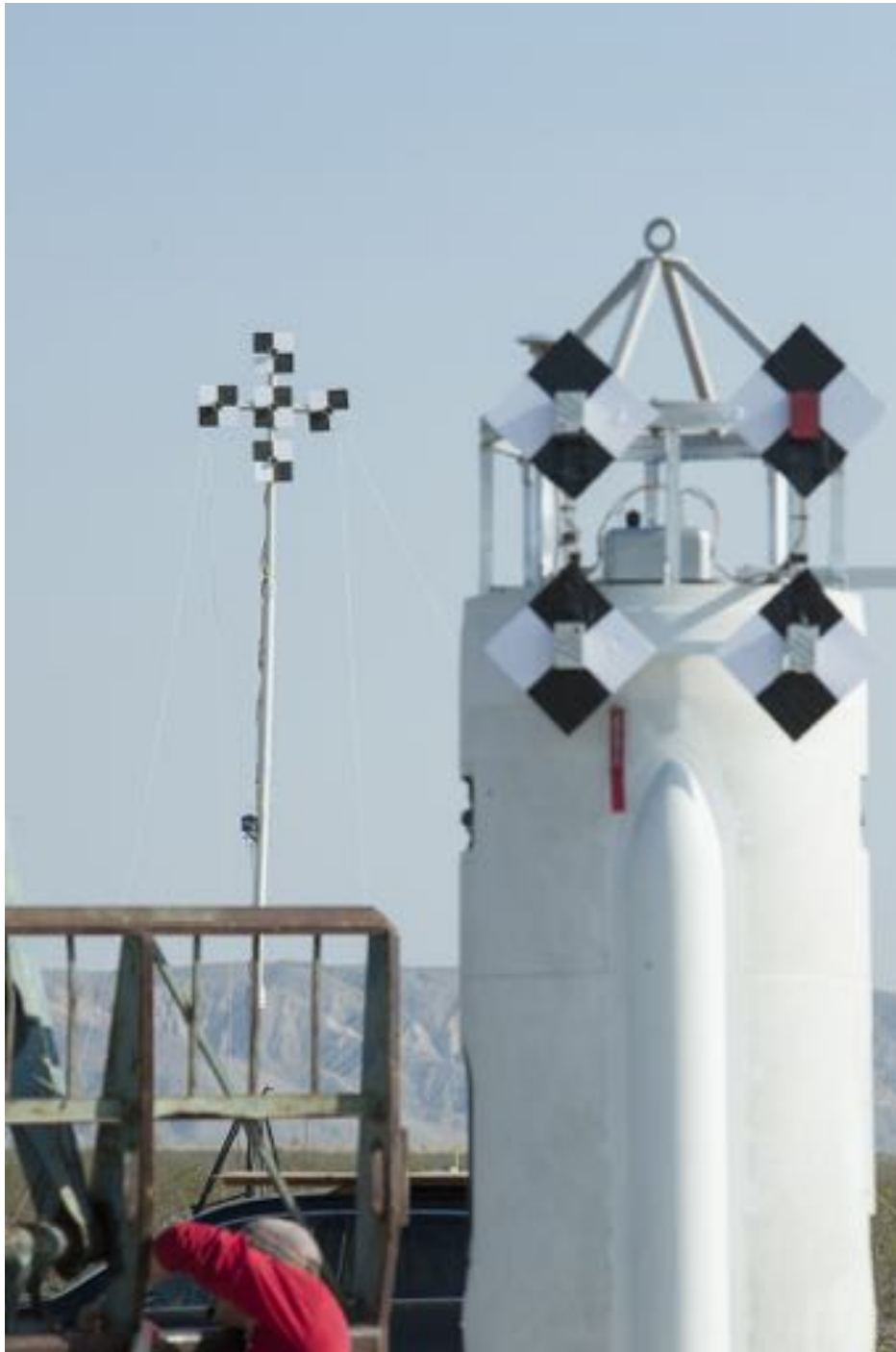
Figure 4.9: Image of background target, with payload on rocket in the foreground. The checkered patterns are used for image recognition to track the position of the rocket relative to the background target during flight.
