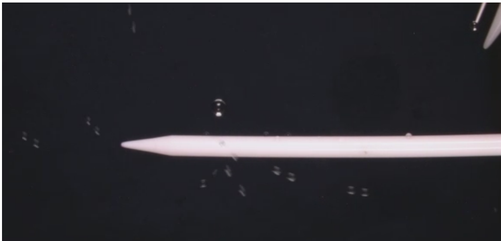
Figure 2.13: Orbital motion of water droplets on the ISS by Coulomb interaction
