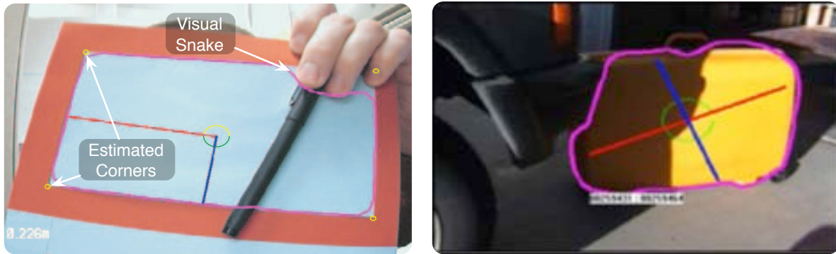
(a) Visual Snake Tracking a Partially Obscured Tar- (b) Visual Snake Tracking a Yellow Suitcase Out- get and Estimating Corner Locations 36 doors with Severe Lighting Variations 35
