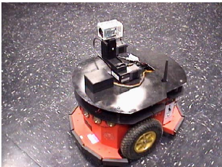
Figure 2.3: ActivMedia Robotics Pioneer 3-DX Robotic Ground Vehicle with a Digital Camera System on a PTU.
