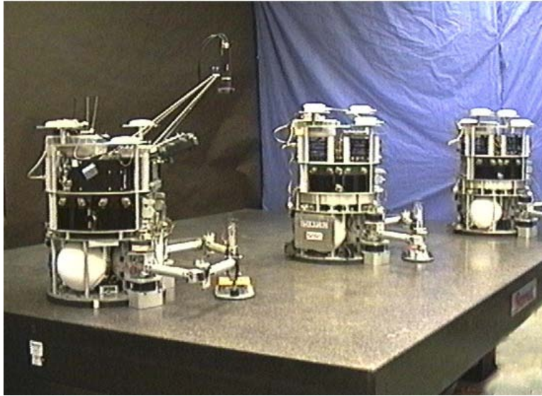
Figure 1.1: Simulated Spacecraft Hovering on a Polished Granite Table at Stanford University's Aerospace Robotics Lab. 14
