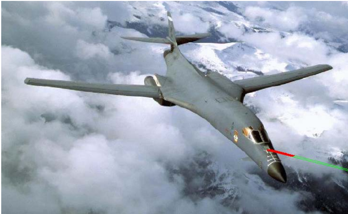
Figure 7.7: Exaggerated Illustration of the Shape of the Range (Red) and Heading Errors (Green) from Aerial Refueling Visual Position Sensing Simulation.
