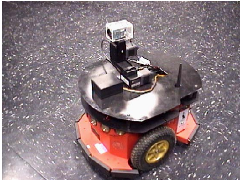
Figure 1.3: Pioneer 3-DX Robotic Ground Vehicle Used for Relative Motion Simulation at the Virginia Tech AVS Lab.
