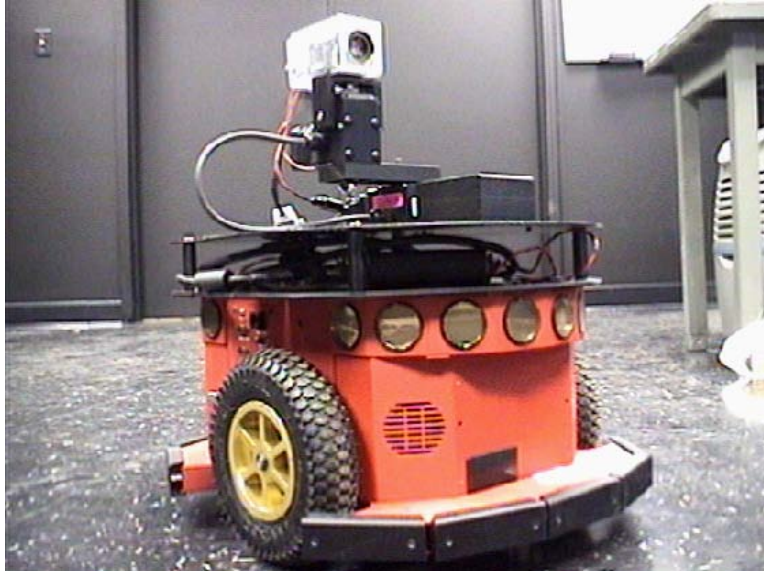
Figure 2.5: PTU Mounted on the Pioneer 3-DX UGV.
