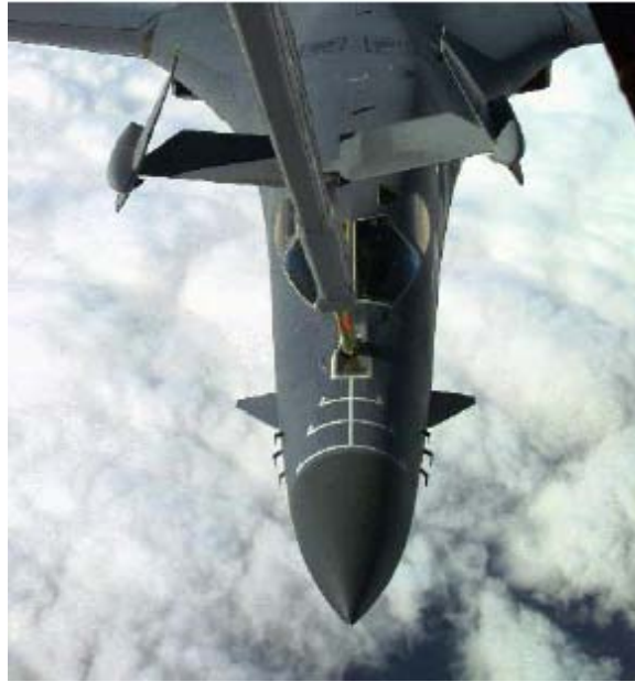
Figure 7.2: Flying Boom Aerial Refueling Method
