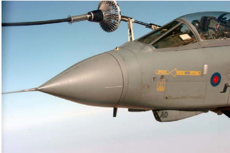
Figure 7.1: Illustration of Probe-and-Drogue Aerial Refueling Method
