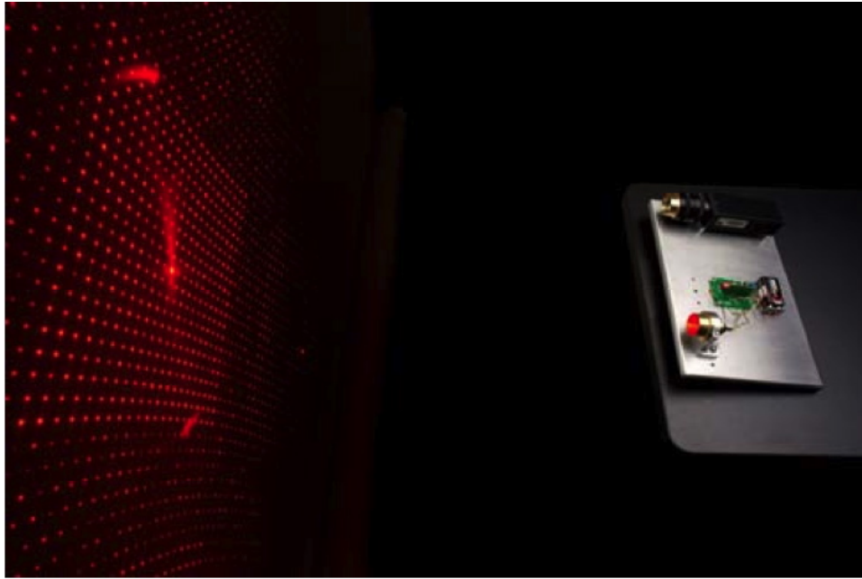
Figure 1.6: JPL Micro-Inspector spacecraft structured light pattern [28]. Courtesy NASA/JPL-Caltech.
