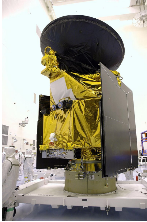
Figure 6.10: Mars Reconnaissance Orbiter wrapped by MLI prior to launch. 5
